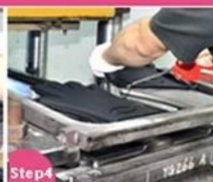
Step4 Vulcanizing and Shaping
