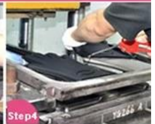
Step4 Vulcanizing and Shaping
