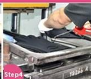
Step4 Vulcanizing and Shaping
