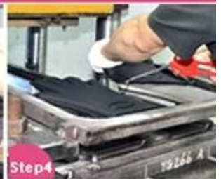
Step4 Vulcanizing and Shaping
