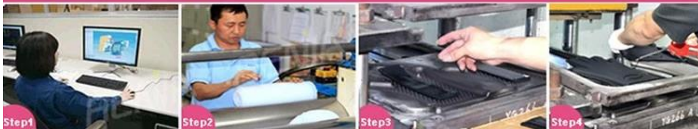
Step1 3D drawing Step2 Material mixing and cutting Step3 Material placing Step4 Vulcanizing and Shaping
