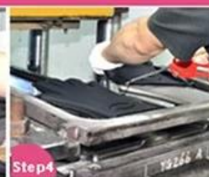
Step4 Vulcanizing and Shaping
