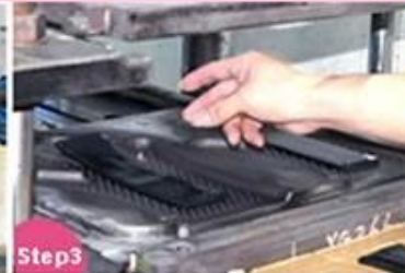
Step3 Material placing
