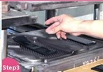
Step3 Material placing
